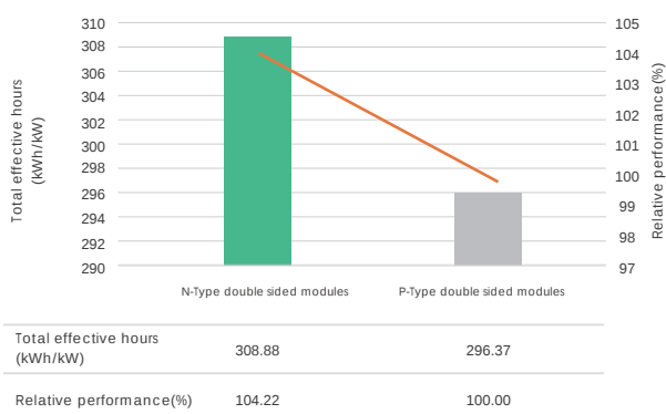
Figure 1. Comparison of the power generation performance of N-type double-sided modules and P-type double-sided modules
